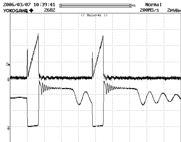
Figure 17 – 265 VAC, Full Load Upper: I_{DRAIN} , 0.2 A / div. Lower: V_{DRAIN} , 200 V / div.
