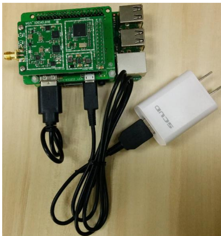
Figure 5 Connect USB Cables
