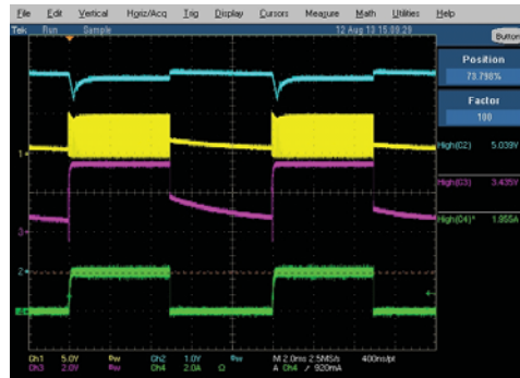
Figure 26. 100 Hz PWM dimming function
