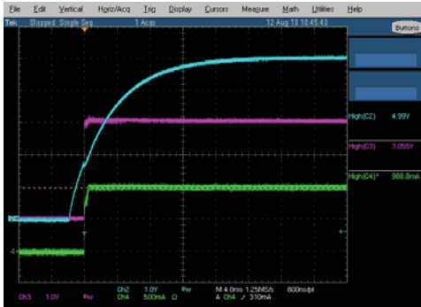
Figure 27. Startup 5 V_{IN} LED 1 A
