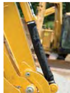
DWN is perfect for protecting hydraulic pistons in harsh environments.
