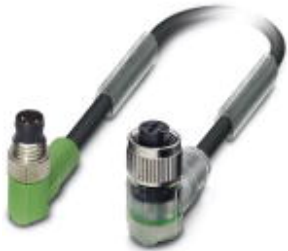
Sensor/actuator cable, 3-position, PUR halogen-free, black-gray RAL 7021, Plug angled M8, on Socket angled M12, A-coded, with 2 LEDs, cable length: 3 m
