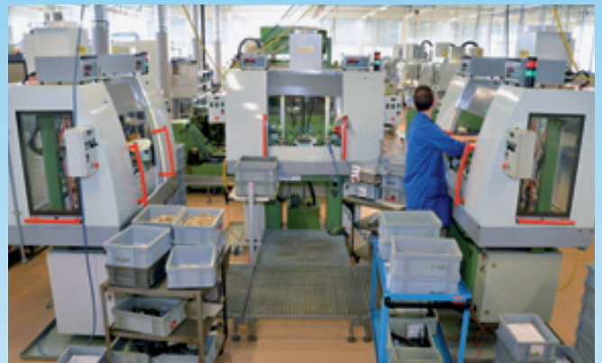
Automatic reworking of female contacts
