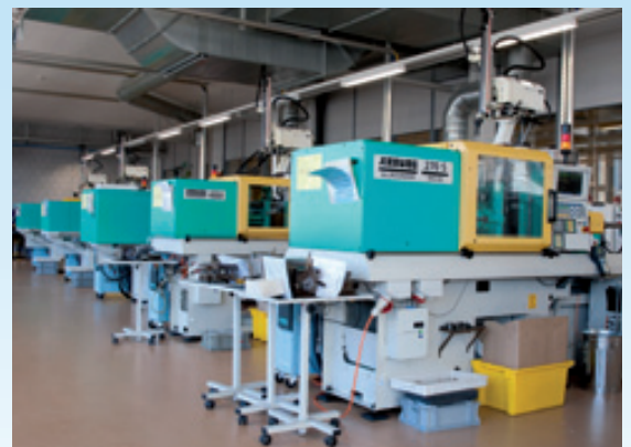
Injection of insulators
