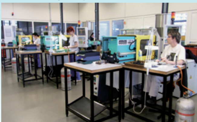
Plastic moulding of bend reliefs
