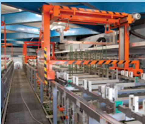
Surface treatment, chrome plating
