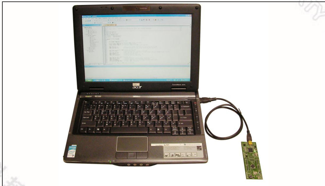
Figure 3-1 NuTiny-SDK-M058S Hardware Setup
