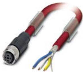
Bus system cable, CC link (10 Mbps), 4-position, PVC, red, shielded, free cable end, on Socket straight M12, A-coded, cable length: 2 m
