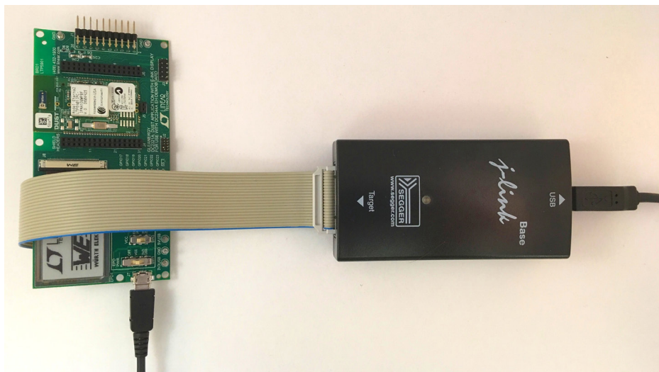
Figure 9b. JTAG Connection with Standard Connector (Not Populated, See BOM)
