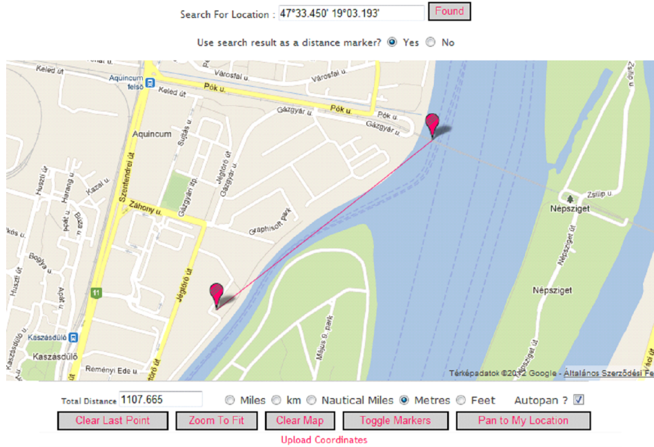
Figure 110. Figure 7.15. Outdoor range test result with two identical printed meander monopole antennas with the 4060-PCE10B868 Pico Board driven by the MSC-LCDBB930-AES Wireless Motherboard
