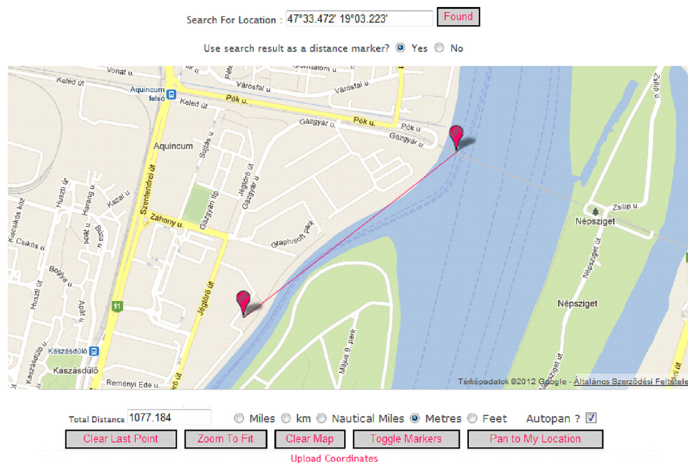
Figure 15. Outdoor range test result with two identical medium size printed ILA antennas with the 4060-PCE10B868 Pico Board driven by the MSC-LCDBB930-AES Wireless Motherboard
