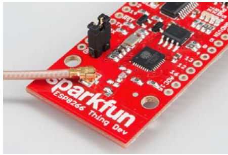
Antenna-select jumper set to U.FL, and an external attached.
