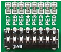
Figure 6-2: Tri-state DIP switch on PORTE
