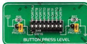
Figure 6-5: Button press level DIP switch (tri-state)
