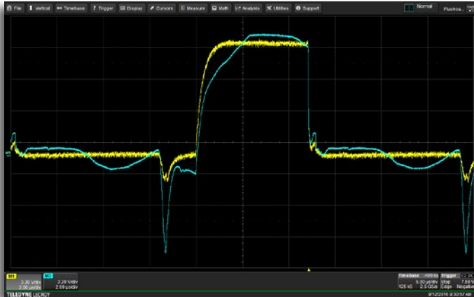
The HVFO (yellow trace) and a conventional HV differential probe (blue trace) capture an upper-side gate drive signal. The HVFO exhibits a classic, textbook shape while the HV differential probe has more loading and lower-side device high dV/dt signal interference.
