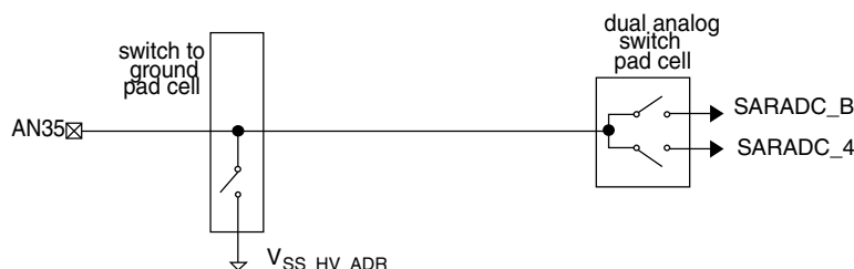
Figure 38-11. Analog input AN35 — discharge switch to AVSS
