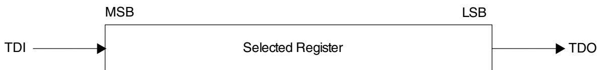
Figure 5-3. Shifting data through a register
