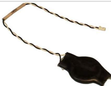
Figure 10. VL-CBR-0203 Latching Battery Module
