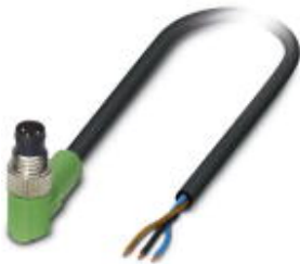
Sensor/Actuator cable, 3-position, PVC, Black RAL 9005, Plug angled M8, on Free cable end, Cable length: 2 m
