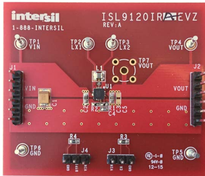
FIGURE 4. ISL9120IRA-EVZ EVALUATION BOARD
