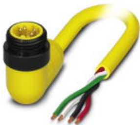
Power cable, 4-position, PVC, yellow, Plug angled 7/8"-16UNF, A - standard, on free cable end, A - standard, cable length: 5 m
