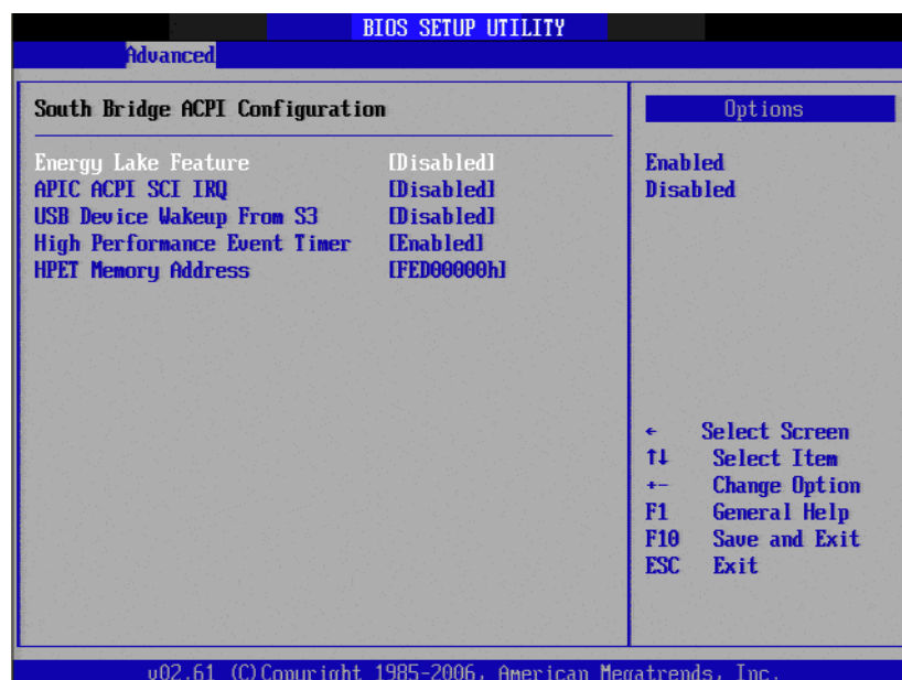
Figure 3.11 Chipset ACPI Configuration
