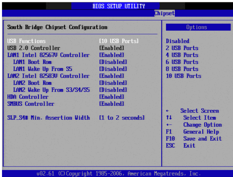
Figure 3.26 South Bridge Configuration
