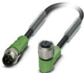
Sensor/actuator cable, 4-position, Variable cable type, Plug straight M12 SPEEDCON, A-coded, on Socket angled M12 SPEEDCON, A-coded, cable length: Free input (0.2 ... 40.0 m)
