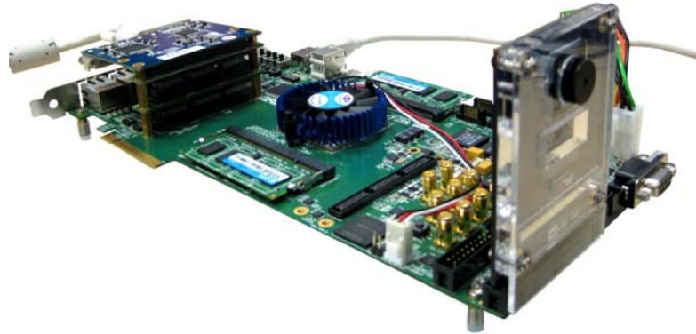
Figure 3.2. The Connection Setup for DE4 users
