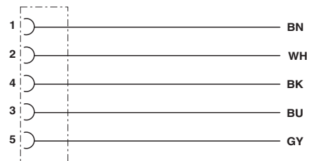
Contact assignment of the M12 socket
