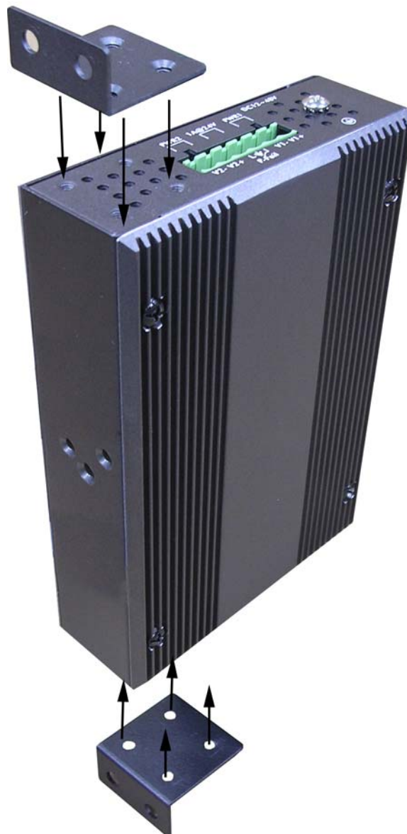
Figure 2.5: Combine the Metal Mounting Kit
