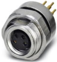
Sensor/actuator flush-type connector, female, 4-pos., M8, rear/screw mounting with M12 thread, with straight solder connection
