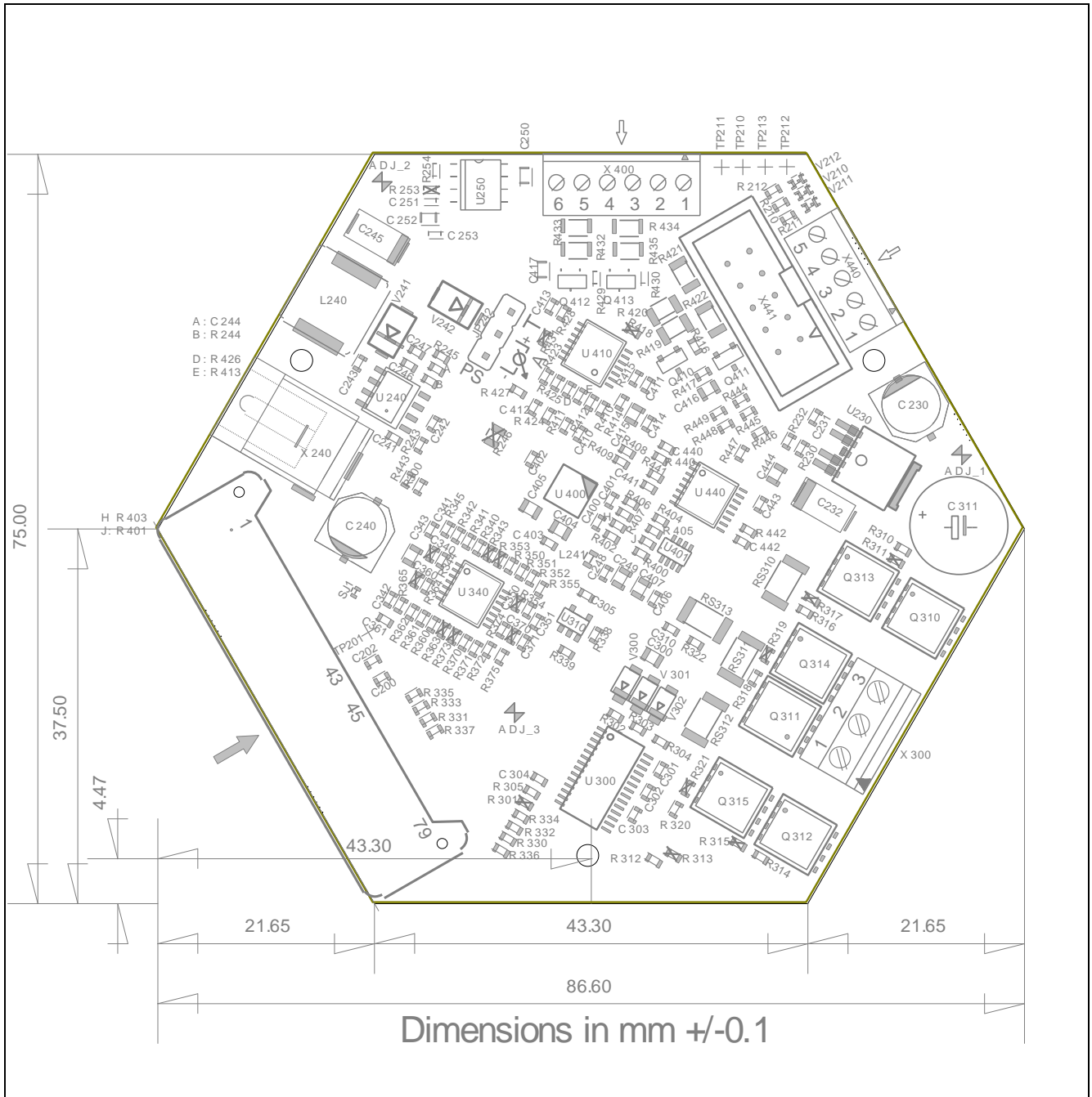
Figure 17 Components Placement and Geometry
