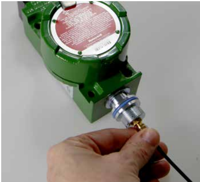
Figure 8. Limitless™ WBX RP-SMA Connection, Remote
