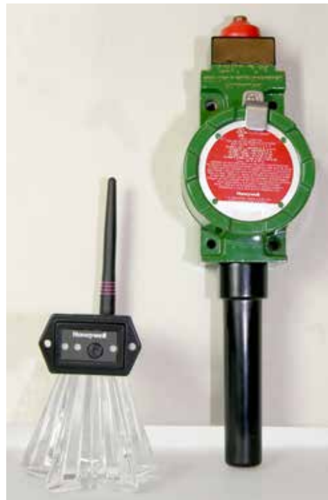
Figure 28. Highest RF Signal When Antennas are as Parallel to Each Other as Possible
