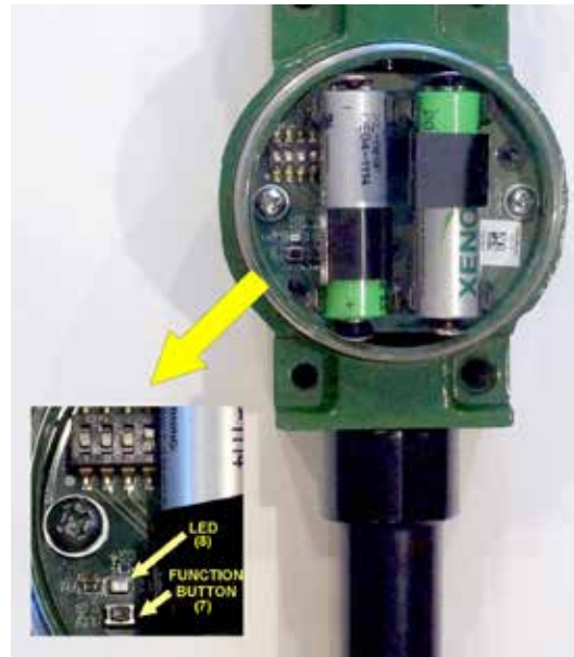
Figure 14. Limitless™ WBX with Function Button and LED
