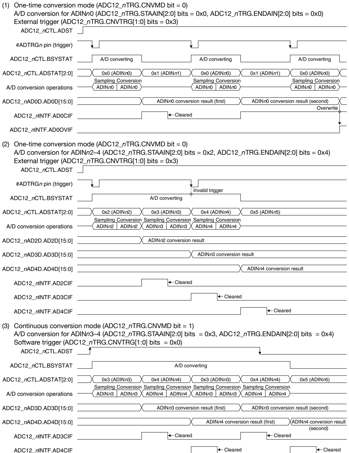
Figure 19.4.4.1 A/D Conversion Operations
