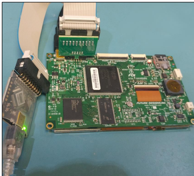
Figure 4: J-Link Connected to \mu EZ GUI
