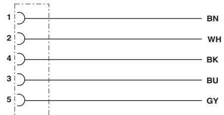
Contact assignment of the M12 socket
