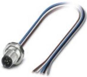
Sensor/actuator flush-type plug, 5-pos., M12, A-coded, rear/screw mounting with Pg9 thread, with 1.5 m TPE litz wire, 5 x 0.34 mm 2
