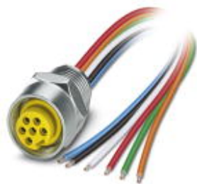
Flush-type connector, 6-position, Socket, straight, 7/8"-16UNF, on free cable end, Front mounting, with 1/2 inch-14 NPT mounting thread, Individual wires, cable length: 1 m
